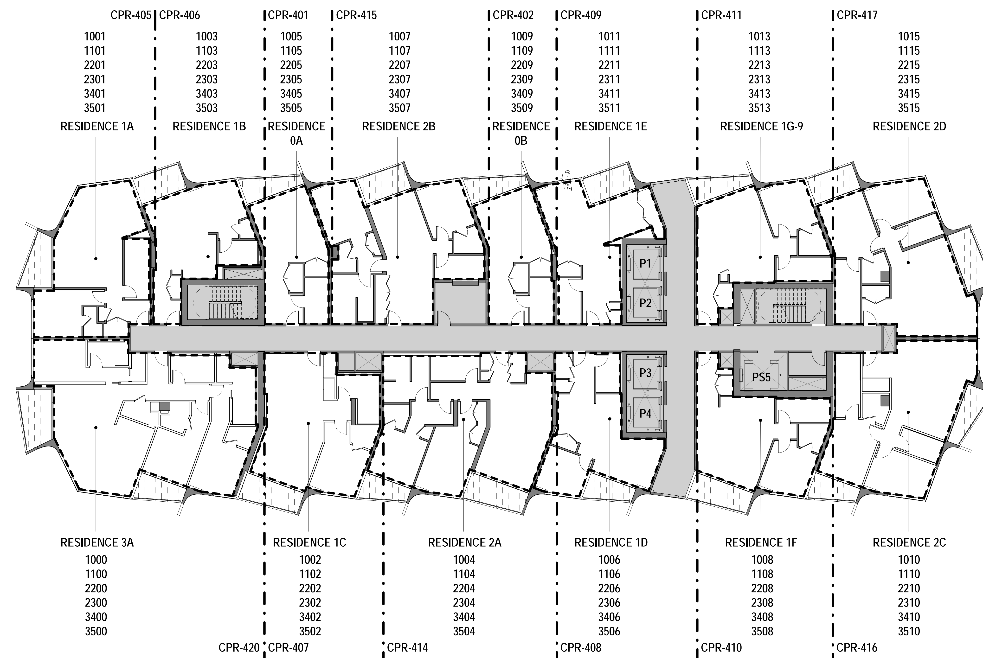
1 FLOOR PLAN TYPE 01 - FLOORS 10, 11, 22, 23, 34, 35 SCALE: 3/32" = 1'-0"
